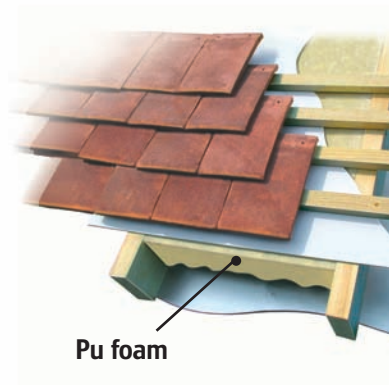
Pitched roof, ceiling at rafter line
