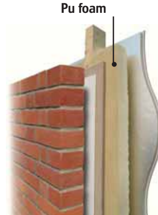
Timber frame wall
